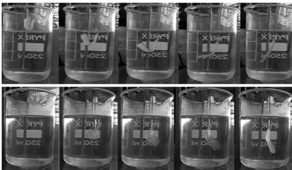
Figure 7 Two sequences of pictures showing shape memory effect for PCO-10 cured with 3% of dicumyl peroxide: first deformation (top) and fourth deformation cycle (bottom).
